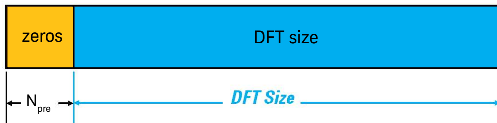
Figure 3(b) Payload OFDM symbol with zeros prefix
