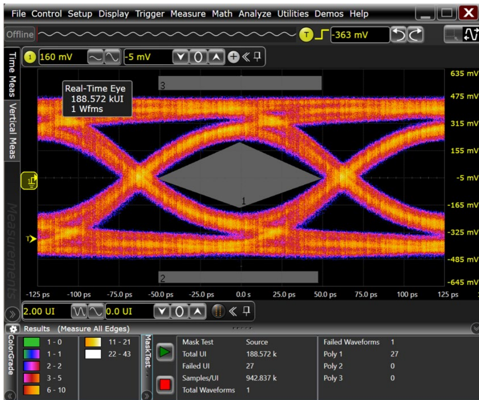
Figure 21. The Serial Data Analysis and optional D9120ASIA Equalization applications allow for the equalization of impaired 8 and 16 Gb/s signals so a clock can be recovered and mask testing can be performed on your waveforms
